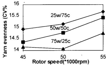
**Figure 1. Yarn evenness for three wool/cotton blends at different rotor speeds**
