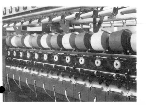
In order to give some description of the naturally brown cotton, we decided to rotor spin it with alternate positions of white fiber for the photo at left. While the black and white picture does not present true color, it does give an interesting contrast. Both cottons were spun with equal efficiency.
